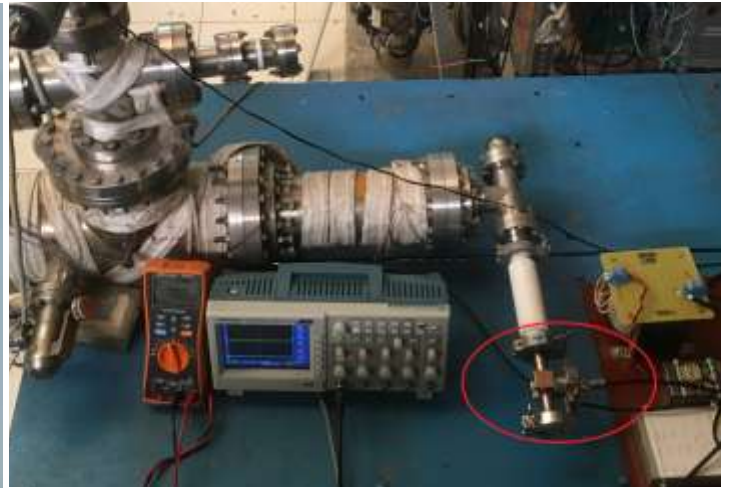
(L) The miniature Penning Ionization Gauge (R) The gauge being tested on an experimental stand.
