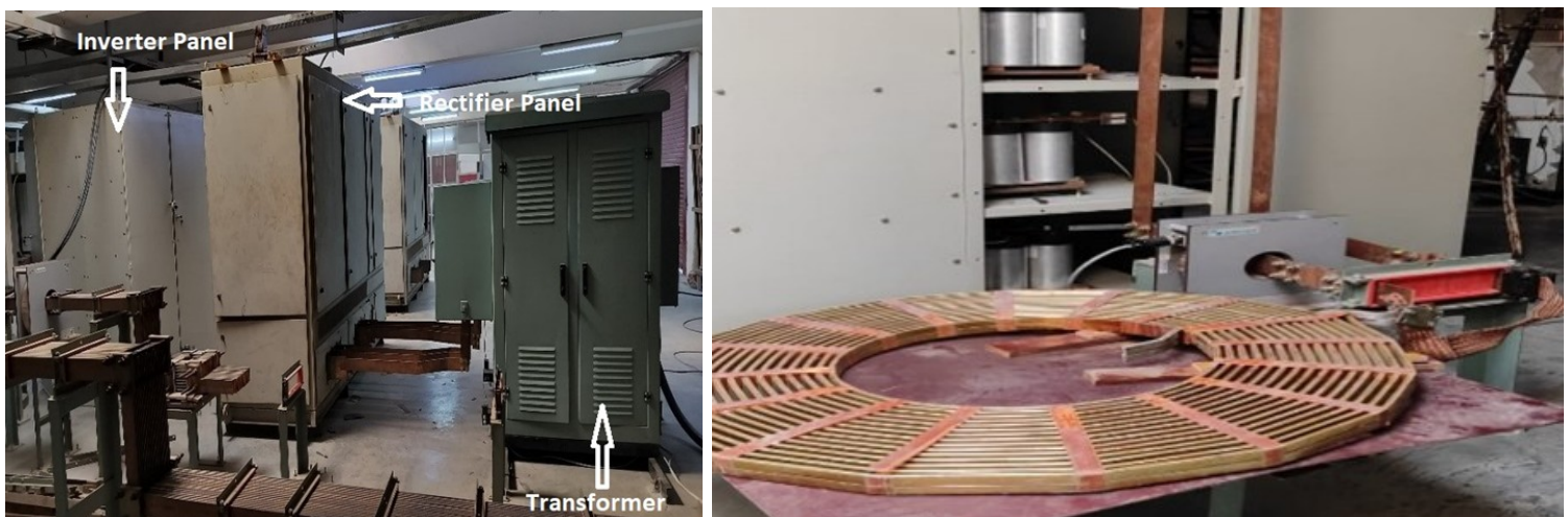
(L) Power Supply with the Inverter Panel, Rectifier Panel and Transformer (R) The Power supply connected to dummy load
