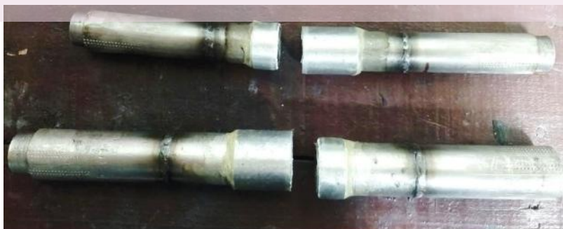
(L) SS-Al bi-metallic joints (R) SS-Al bi-metallic joint after tensile pull test
