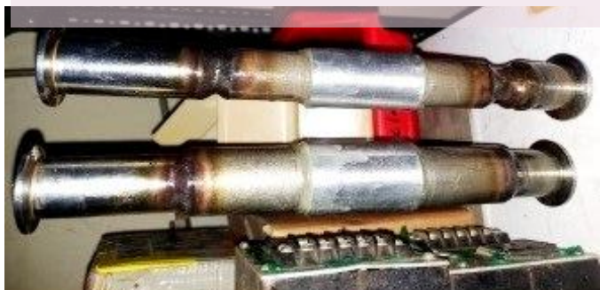
(L) SS-Al bi-metallic joints (R) SS-Al bi-metallic joint after tensile pull test
