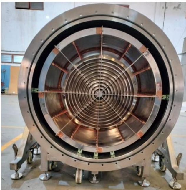
(L) Fabricated Cryopump showing internal geometries (R) Assembly of the LCTF at Factory
