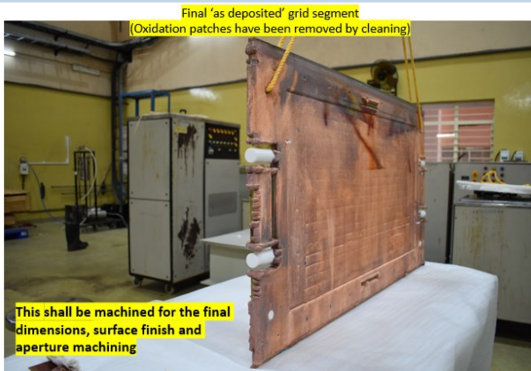
Electrodeposited Grid segment (as deposited condition)
