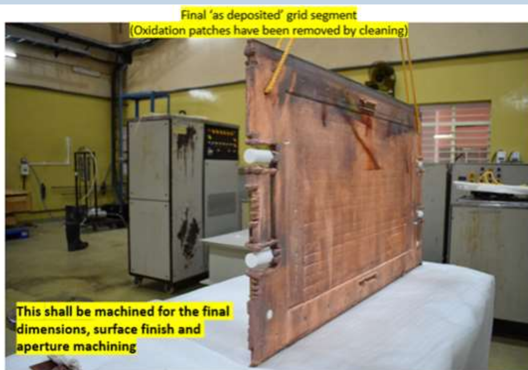
Electrodeposited Grid segment (as deposited condition)
