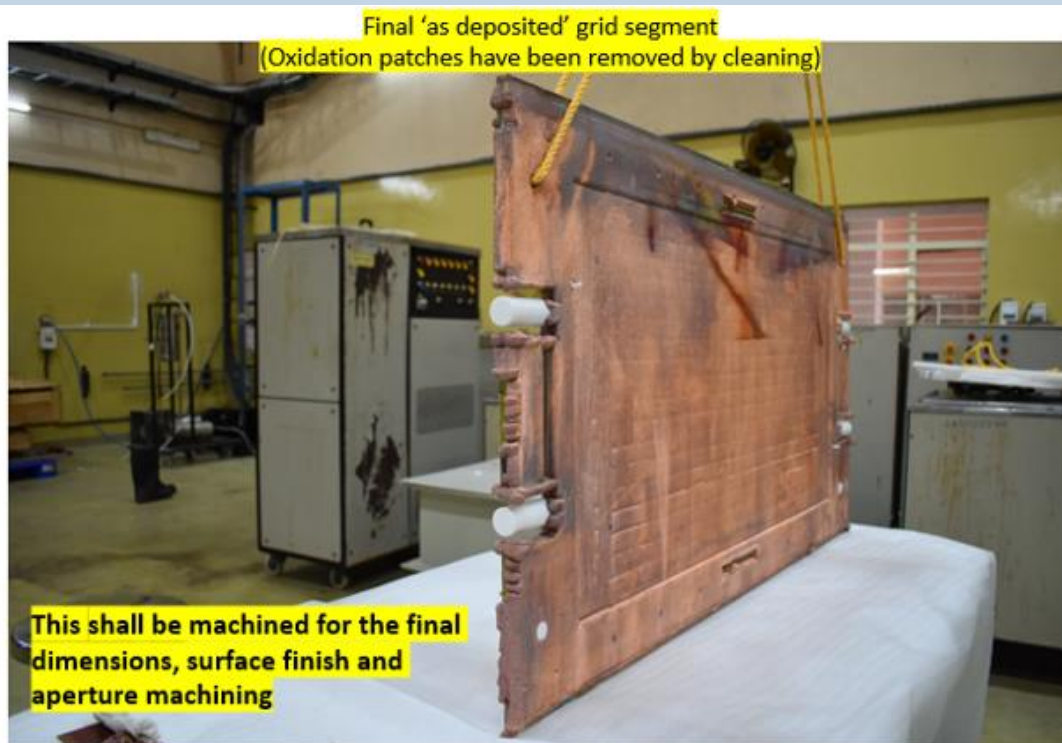
Electrodeposited Grid segment (as deposited condition)
