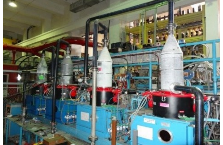
Figure-2: HP LHCD source system, comprising of four klystrons, each rated for 0.5MW-CW RF power at 3.7 GHz
