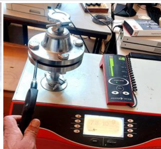
Helium leak test
