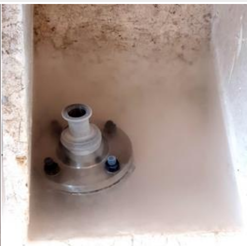
Thermal cycle test at 77 K
