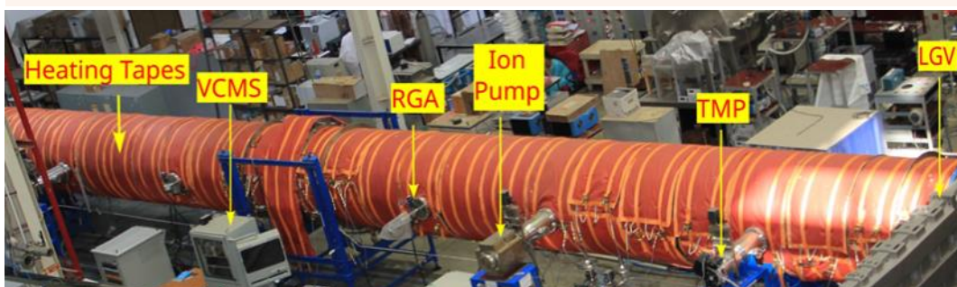
Integrated Vacuum Vessel (IVV) post assembly
