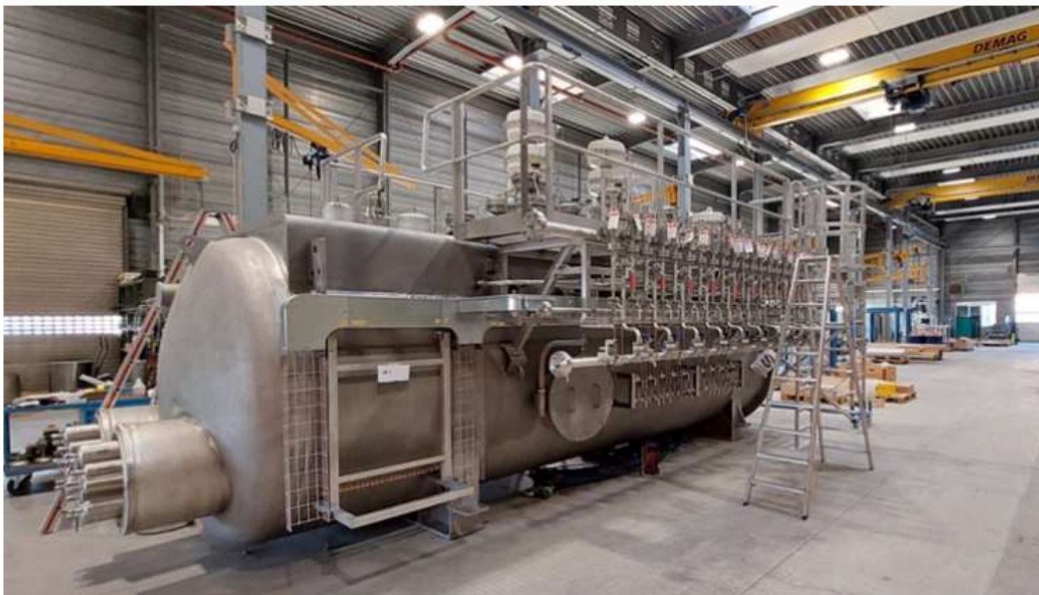
Figure shows the Thermal Shield Cold Valve Box at the workshop during Factory Acceptance Test
