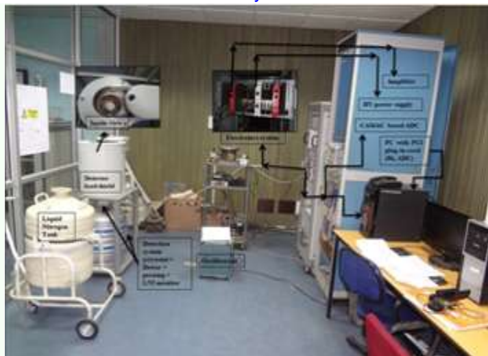
Fig. 3 Experimental set-up of off-line gamma ray spectroscopy
