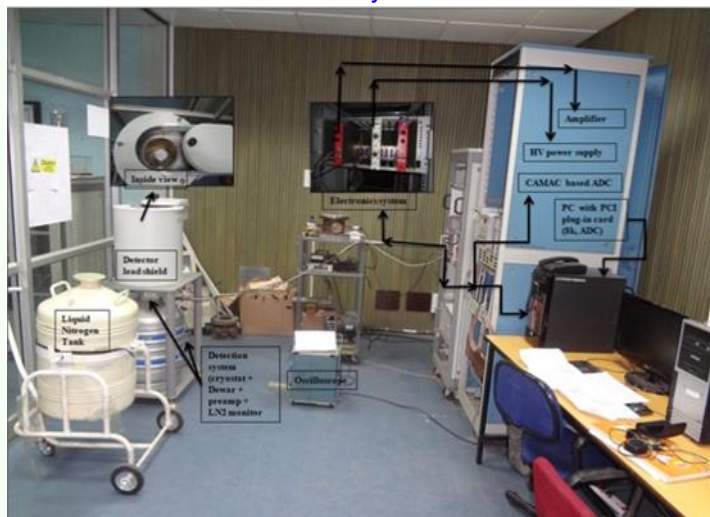
Fig. 3 Experimental set-up of off-line gamma ray spectroscopy
