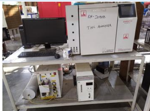
GC for PPB level oil measurement in helium gas
