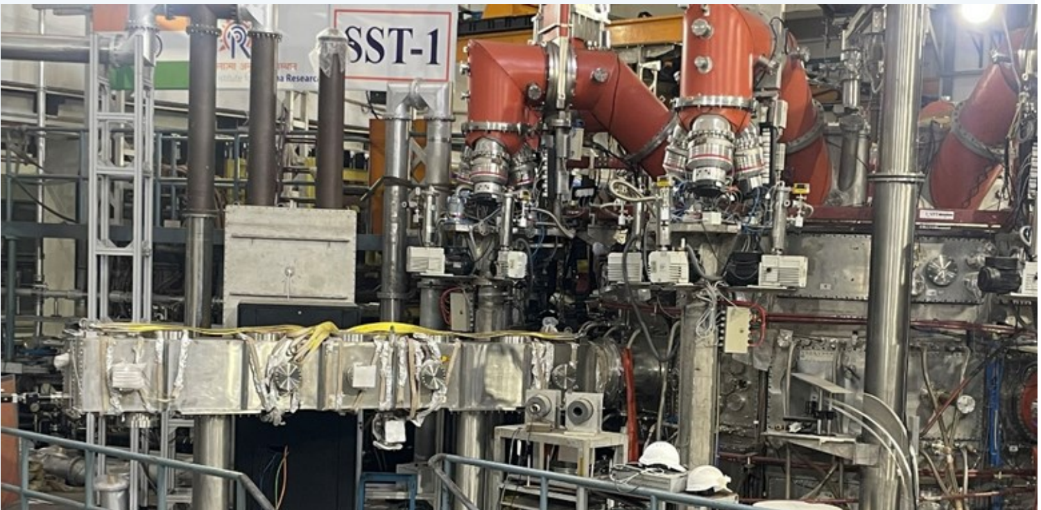
IVIS Mounted at Port #7 of SST-1 VV
