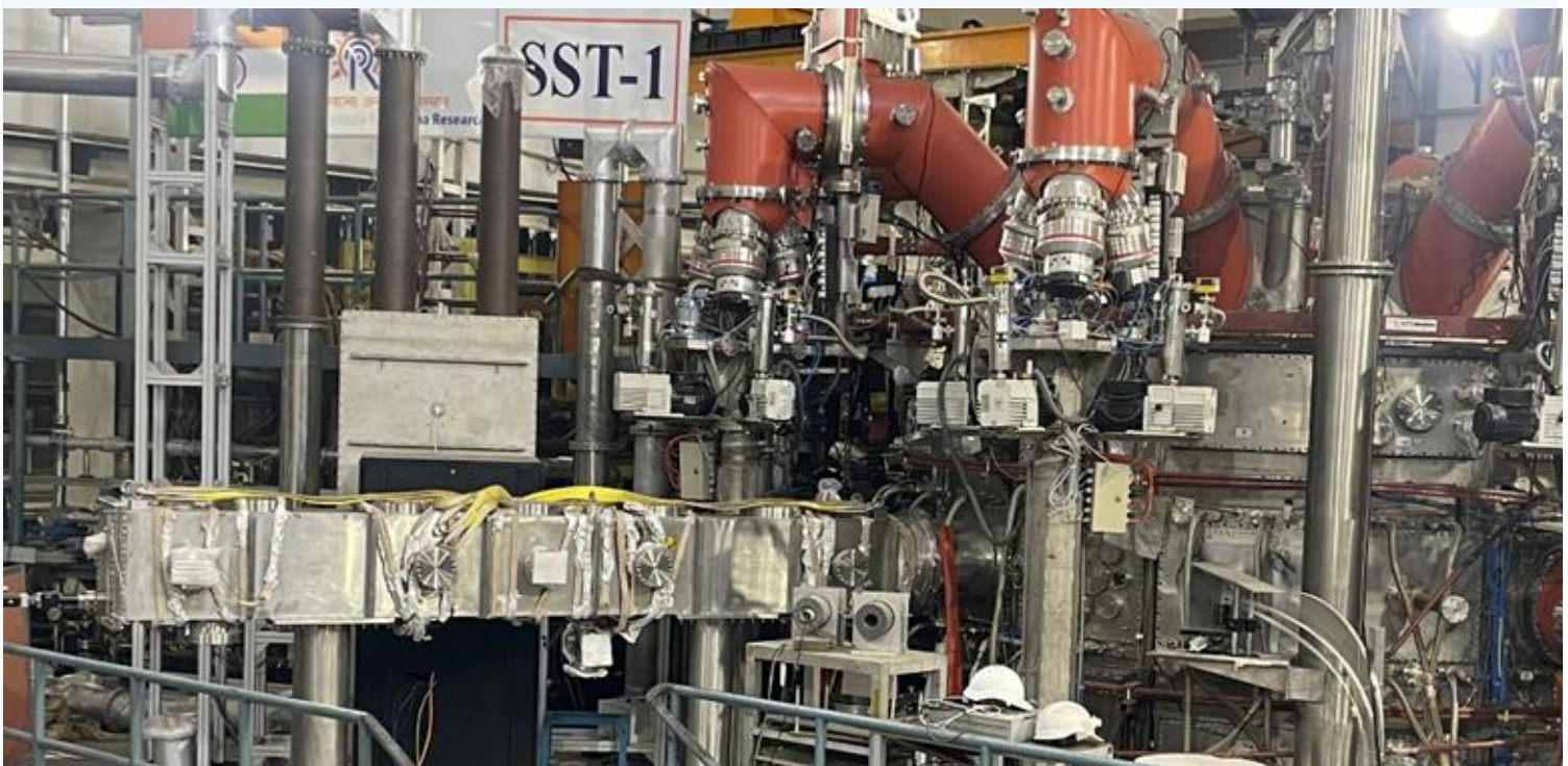
IVIS Mounted at Port #7 of SST-1 VV
