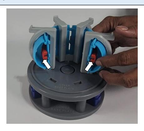
Snap-fit the two vacuum vessel blocks to assemble the TF and vacuum vessel. Slide the remaining two TF coils on to the third vacuum vessel assembly and snap-fit the TF coils to the base. Then proceed to snap-fit the third vacuum vessel to the remaining two previously assembled vacuum vessels.
