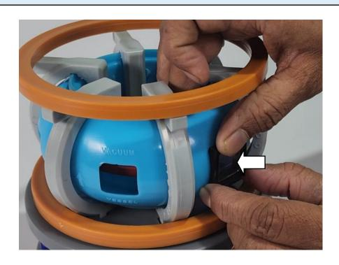
Take the Central Solenoid block and push-fit it on to the groove provided on upper base plate, in the vertical centre of the device.
