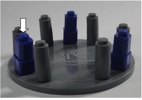
Take the upper base plate and push fit it on to the support system and vacuum pump blocks mounted on the lower base plate. Some amount of adjustment will be needed to align all the stubs. Once aligned, push fit all the parts into position.
