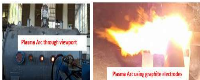
Figure A.1.5: 100kW plasma arc system.
