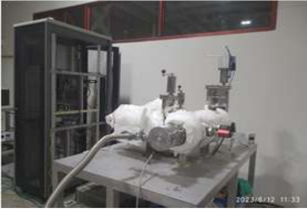
Figure B.2.1: Outgassing measurement set up.
