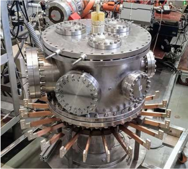
Figure A.2.7: Newly fabricated SMARTX-C vacuum chamber along with toroidal field coil bus-bars, and support structure.
