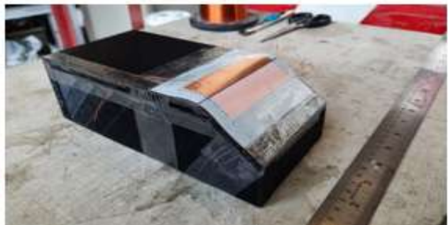
Figure A.1.23: Scaled up models of Ahmed body and automobile.
