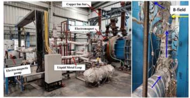
Figure A.4.6: Pb-Li MHD loop at the institute (left) and 'U' shaped circular cross-section test mock up inside the magnet pole gap (right).
