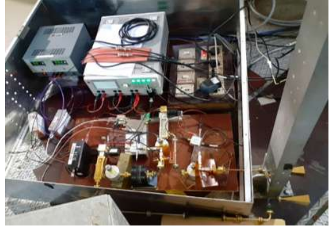
Figure A.3.11: Schematic block diagram and 100 GHz heterodyne system.
