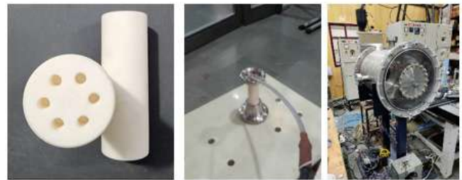
Figure A.4.20: Development of post insulators with insulator metallic flange bolted concept and HV testing.
