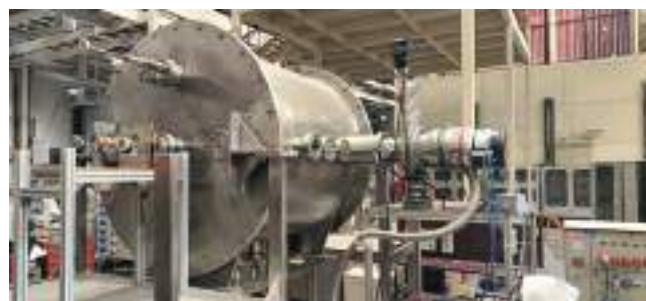
Figure A.1.16: Large Helical Thruster System with installed plasma source, helicon antenna.
