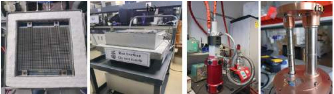
Figure A.3.21: (a) Black body calibration source, (b) Closed loop dry cryogenic detection system.
