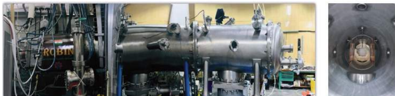
Figure A.4.19: Upgraded ROBIN test bed with additional chamber; inside view of the beam line with neutralizer and ERID mounted in the vessel.
