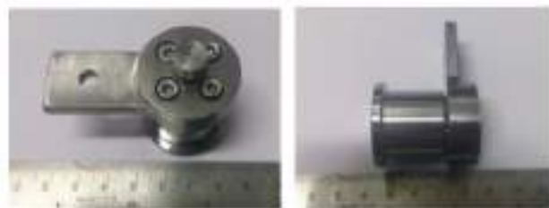
Figure A.4.6: Fixture for shear punch testing of tungsten using Gleeble 3800.
