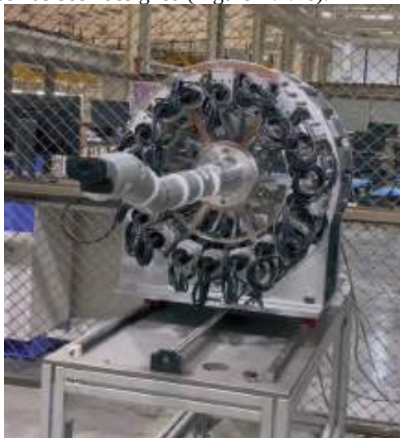
Figure A.4.16: (a)Hyper Redundant Inspection System (HRIS) in operation. (b) UHV Compatible version.
