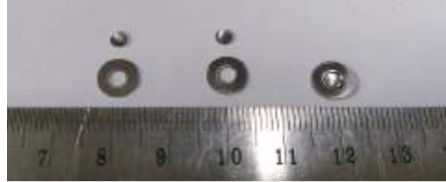
Figure A.4.7: Tungsten samples after shear punch testing.
