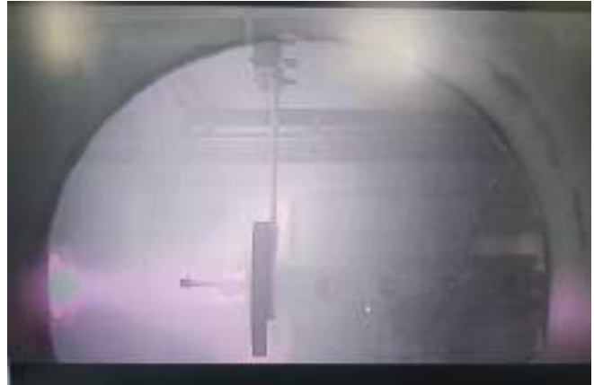
Figure A.1.19: Thrust sensor with plasma plume in thruster chamber.
