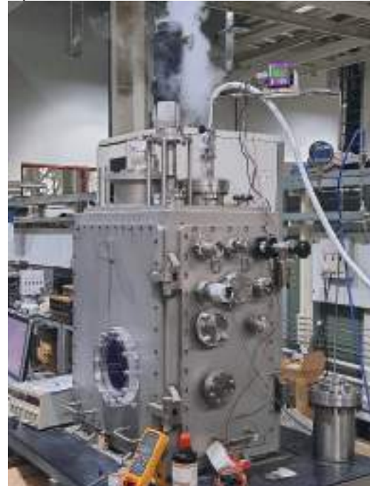
Figure A.4.14: (a) Testing of cryogenic extruder system using gaseous helium (front view).
