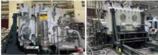
Figure A.4.4: Helium cooled target handling system and extension chamber for High Heat Flux Test Facility (HHFTF).
