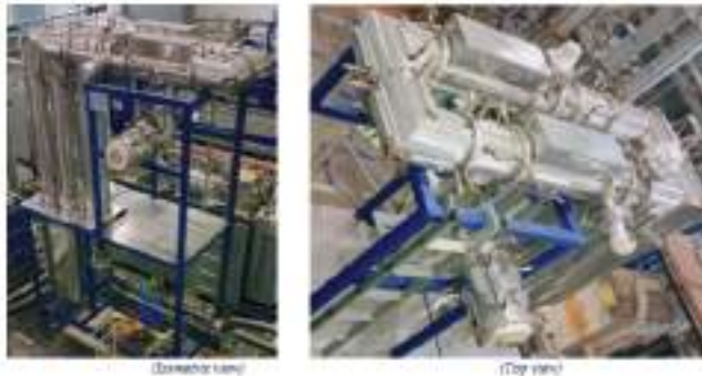
Figure B.1.13: Assembled 3 MW mismatch transmission line.
