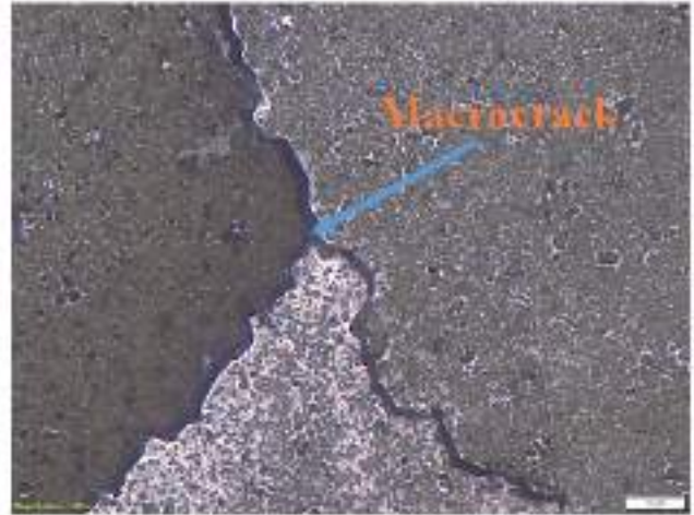
Figure A.4.10: Exposed Tungsten sample for 15 shots of hydrogen plasma.
