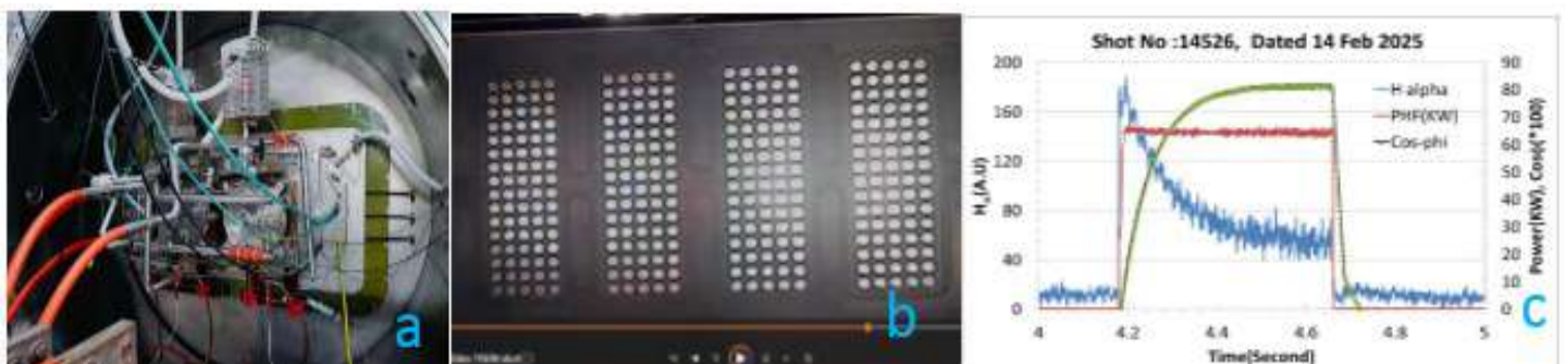
Figure A.2.35: (a) TWIN Source Test Bed (b) TWIN source Plasma; (c) Typical high RF power coupling plasma shots.
