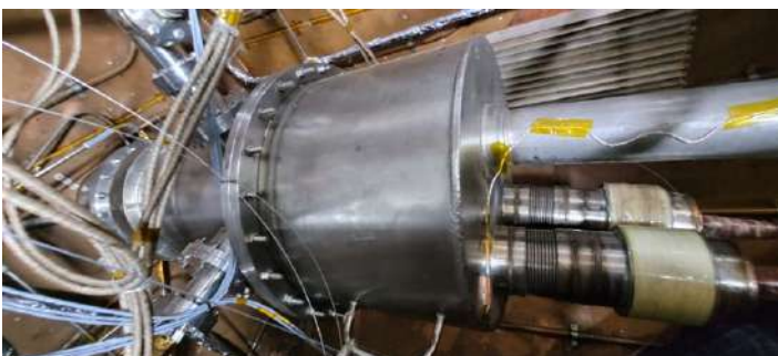
Figure A.1.39: CFS chamber with room temperature radiation components inside the chamber.
