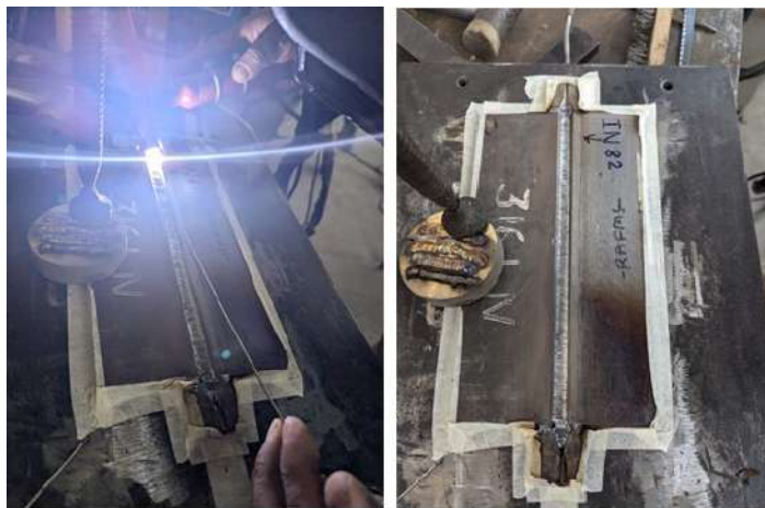
Figure A.2.27: Dissimilar weld joints of IN-RAFM – SS 316LN using INCONEL-82 filler wire.
