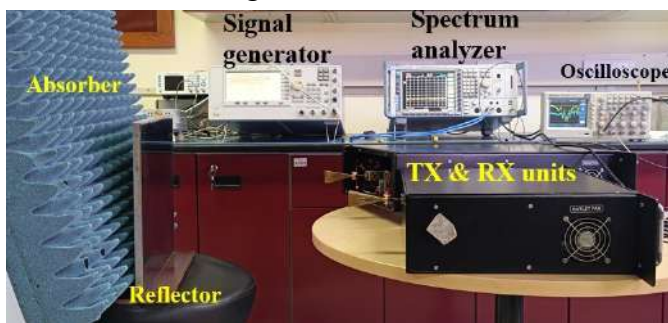
Figure A.1.26: In-lab Characterization set-up for developed W-band trans-receiver unit.
