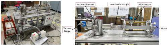
Figure A.2.34: Vacuum automation system.
