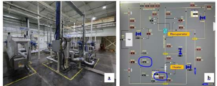
Figure A.2.20: a) Photograph of EHCL system b) Hot testing results of EHCL at 300^\circ\text{C} , 80 bar conditions.
