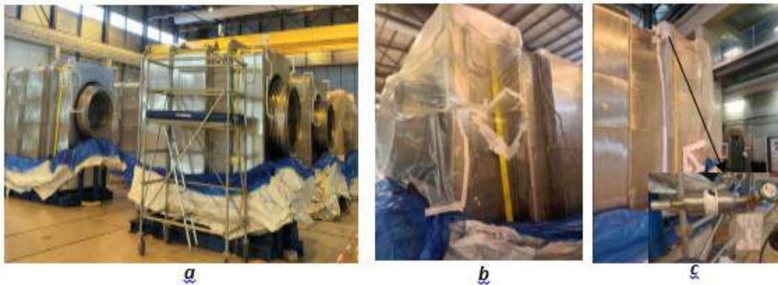
Figure B.1.6: Torus Cryo-Pump Housing and Helium Leak testing of TCPH.
