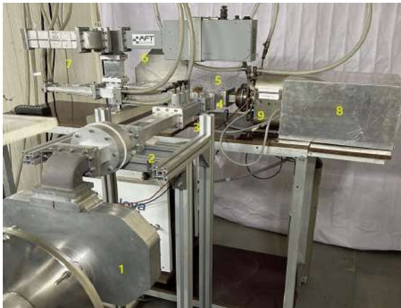
Figure A.3.17: SYMPLE experimental set-up. 1. Mode Converter, 2. DC Break, 3. Stub Tuner, 4. Directional Coupler, 5. Circulator, 6. Variable Attenuator, 7. Dummy Load, 8. Magnetron and 9. Electromagnet.
