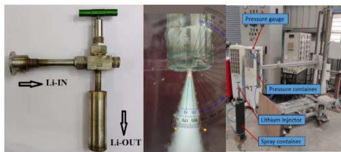
Figure A.2.11: (a) Fabricated and assembled lithium injector (b) Test setup for spray testing of the lithium injector (c) Testing of Li injector to demonstrate dispersed spray pattern
