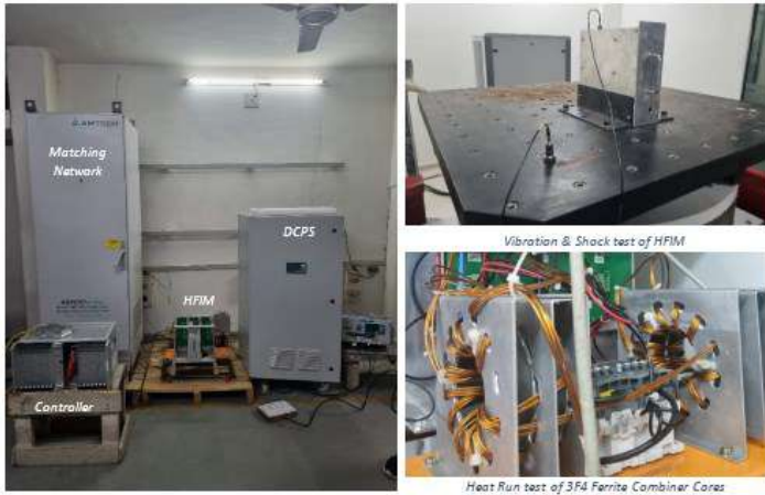
Figure B.1.20: HFIM Testing.
