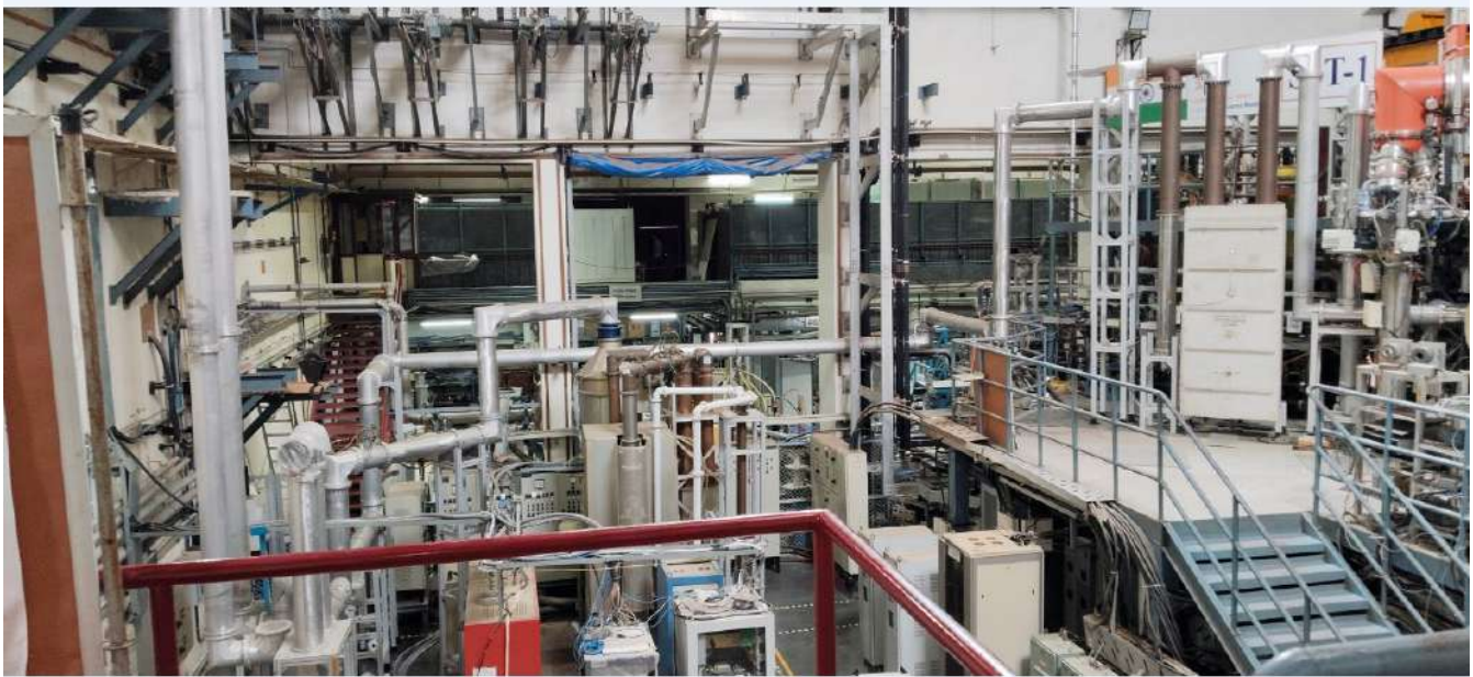
Figure A.1.34: Newly installed Aluminium transmission line and matching network at SST-1.
