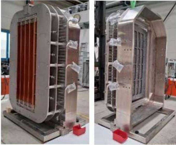
Figure B.1.14: Assembly of 3-grid accelerator (with dummy insulators).
